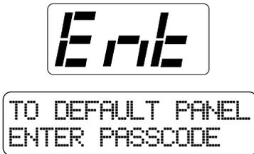
If it is entered correctly, the Control Station will go into a locked out state for a few seconds and then may display the No Communication condition and flash all LEDs before displaying the panel revision and returning to the Ready mode.
