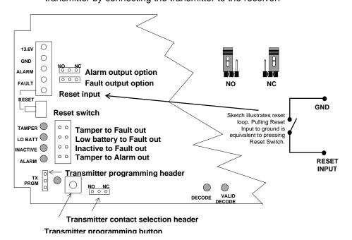
**Power the Receiver:** Apply power and ground to marked terminals.
