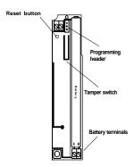
Program contacts: N/O or N/C, as needed not supported by the FA401 Internal contact: Typical battery life: 3 years
