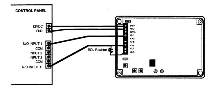
Typical configuration using open collector output of C-404 Reciever. The Panel must accept a normally open device and the common input terminals must be in common with power common.
