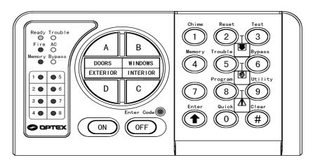
Quad Keys activate preassigned zone groups or preconfigured arming modes. Turn on the security system by selecting the appropriate button and pressing 'On'.
