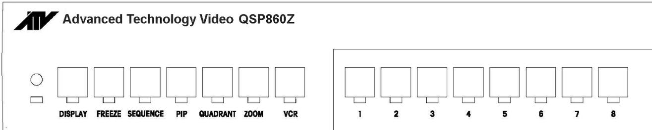
Your QSP-860Z has seven mode control buttons and eight numbered camera buttons which allow easy access to all modes of operation. The seven mode buttons on the left are used to control monitor display operations and VCR playback. An LED below each button will light when the unit is in the mode corresponding to that button.
