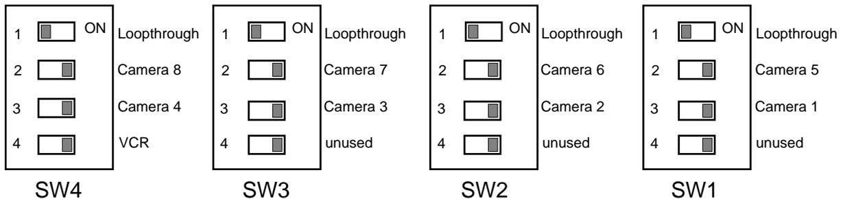
The video line termination switches for each camera input are located in the rear of the unit and are accessed by removing the top cover. The switches are in the order shown above when looking down on the circuit board. The above switches are shown in the factory default settings (75 ohm terminations ON).
