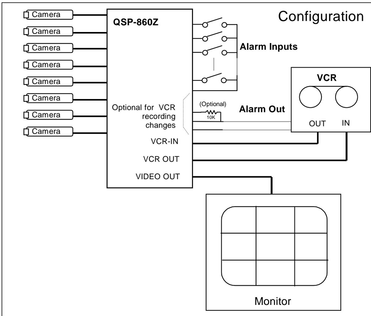
The above diagram shows the typical 8-camera installation for the QSP-860Z. Up to eight cameras can be connected to the dual page real time quad using the back panel connectors.
