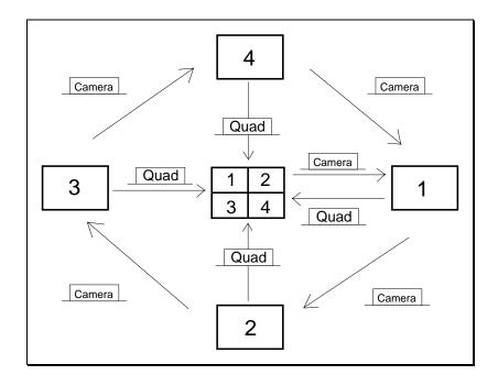
**Quad** Returns the unit to Quad mode regardless of present mode of operation.
