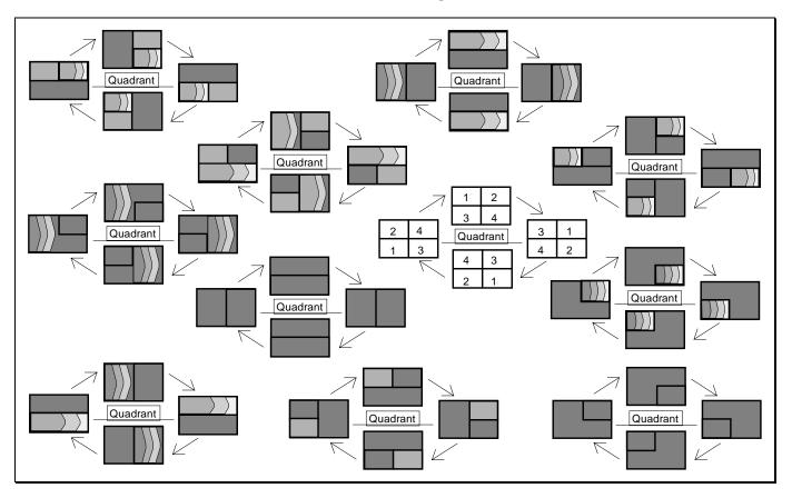
**Quadrant** In any mode with multiple cameras displayed, this button will cause the cameras viewed to rotate clockwise on the screen. This allows the placement of one or two inserts in desired screen locations.
