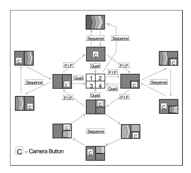
Sequence When starting in the Quad mode, pressing this button causes the unit to switch to "Full Frame Sequencing" mode. Once in this mode, pressing the button toggles the unit back and forth between "Full Frame" and "Full Frame Sequencing" modes. In both single and dual PIP modes and in split screen, pressing this button will enable camera sequencing to switch from one display area of the screen to another.
