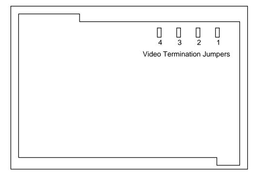
The video line termination jumpers for each camera input are located in the rear of the unit and are accessed by removing the top cover. Jumpers should be removed if camera loop-through is used to forward a camera input to another video switcher or splitter.
