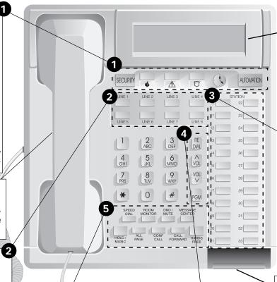
The **Liquid Crystal Display** (LCD) provides system status and will guide you through system and station programming via visual prompts.
