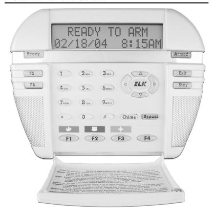
**Fire** - If enabled, this key activates the local fire alarm audibles and reports the alarm to a central monitoring center, if monitoring is included as part of the system. This type of activation is generally programmed for double press or press and hold for 2 seconds.
