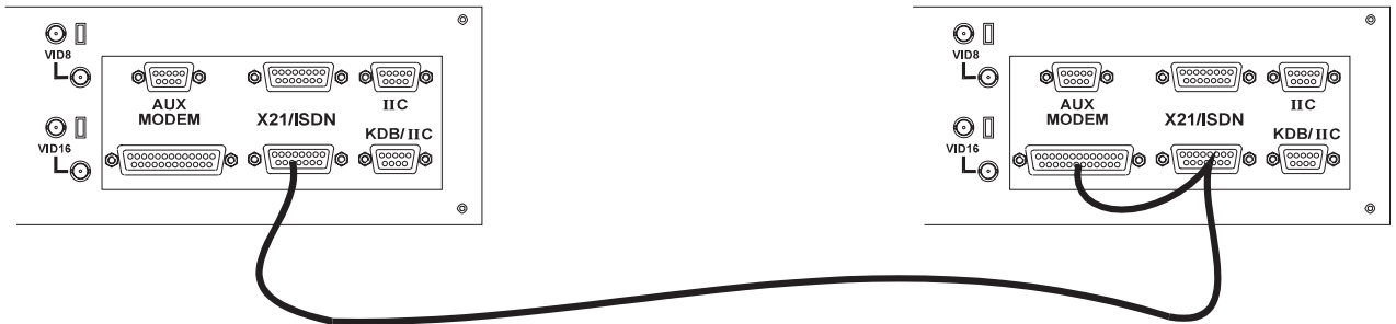
Fig: 9 Demo cable connections
