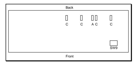
The QSP-441 input option shunts are located in the rear of the unit and the sequence dwell setting DIP switch is located toward the front right hand corner. These are accessed by removing the top cover.
