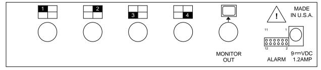
The power connector is for a 9 Volt DC power adapter rated at 1.2 Amps. It is **NOT** recommended that any adapter other than the one shipped with the QSP-441 be used.
