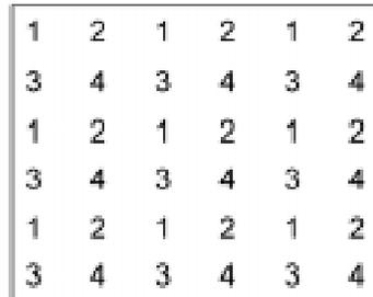
Distribution of detectors for cross alarm in a large open area with 4 zones. For a smaller installation, use any segment of this example
