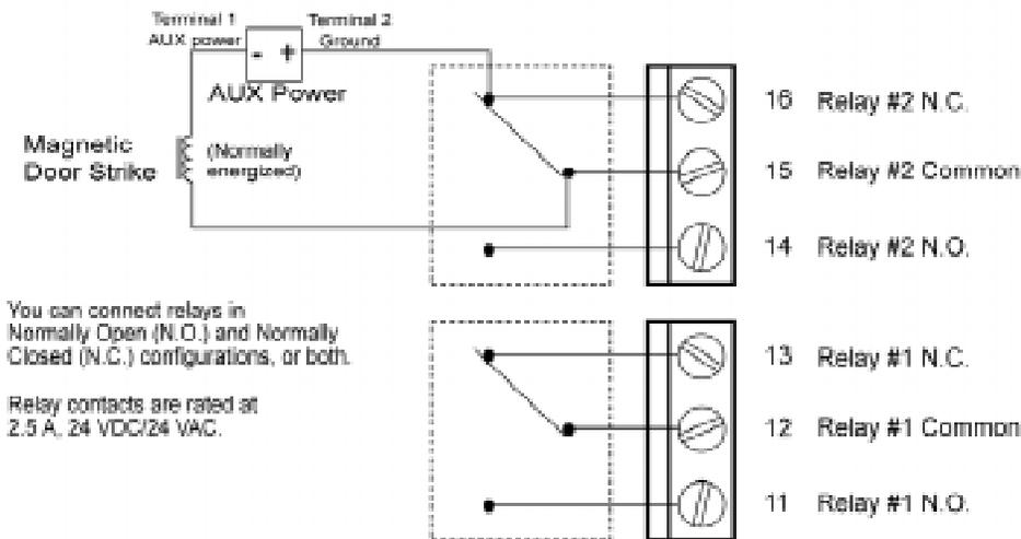
Figure 6-11 Auxiliary Relays
