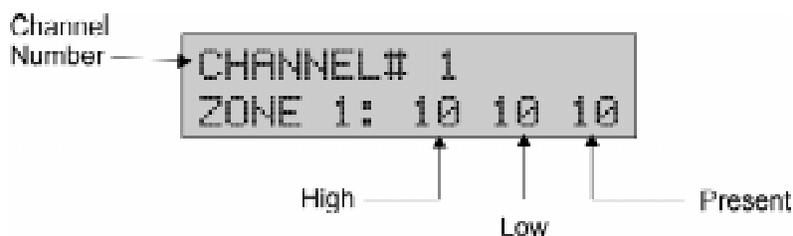
These values, or “step numbers”, are not actual voltage readings. Use the information following these steps and Table 9-1 to determine the values acceptable for each input, and to calculate the actual voltage reading.
