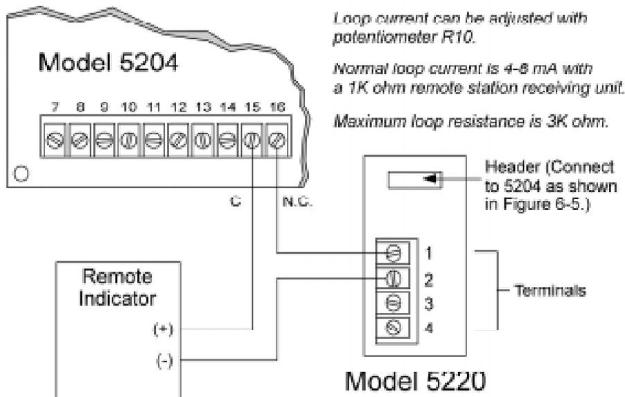
**Figure 6-6 Wiring the 5220 for Polarity Reversal**
