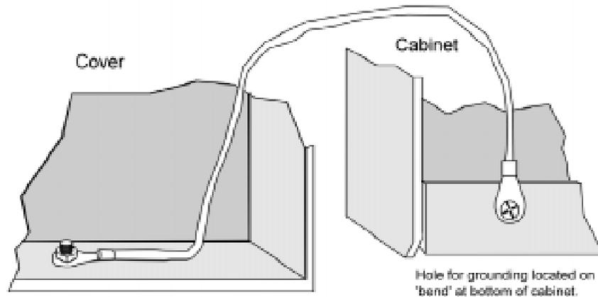
Figure 5-2 Connecting the Ground Wire
