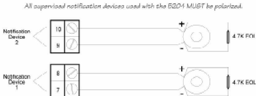
**Figure 6-10 Model 5204 Notification Device Connections**
