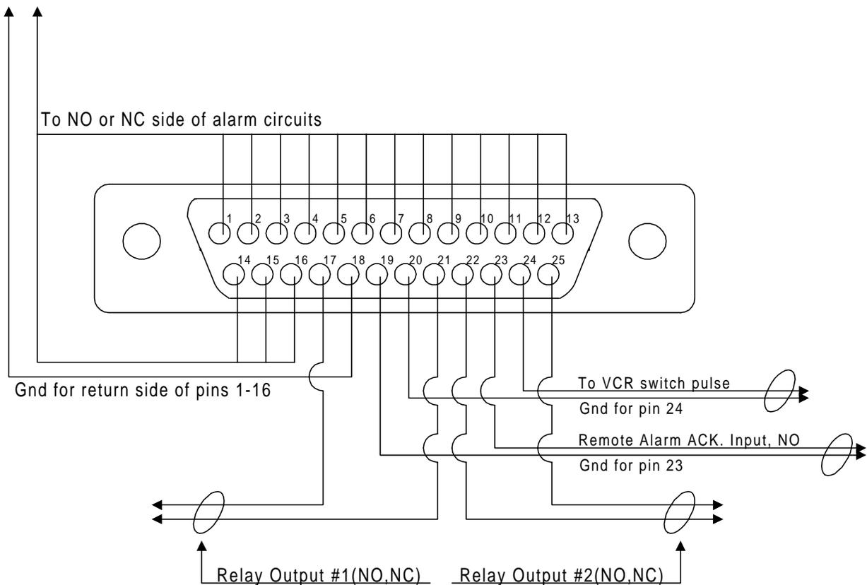
Figure 5. DB-25 Connector Pinouts
