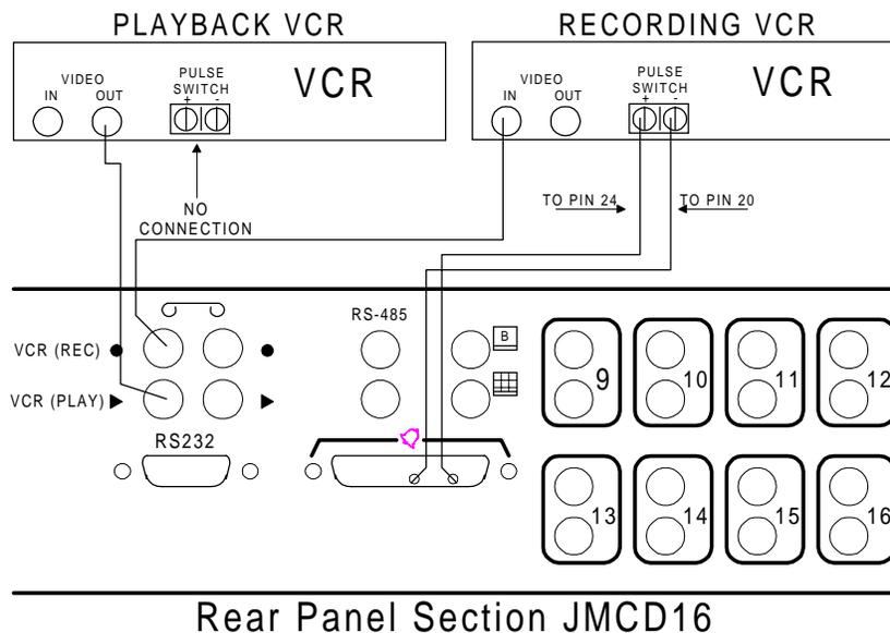
**Figure 3.2 Connecting Two VCRs For Duplex Recording and Playback - JMCD16**
