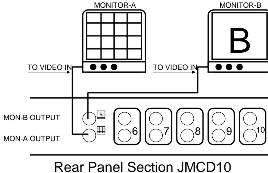
**Figure 2.2 Connecting Monitors - JMCD16**
