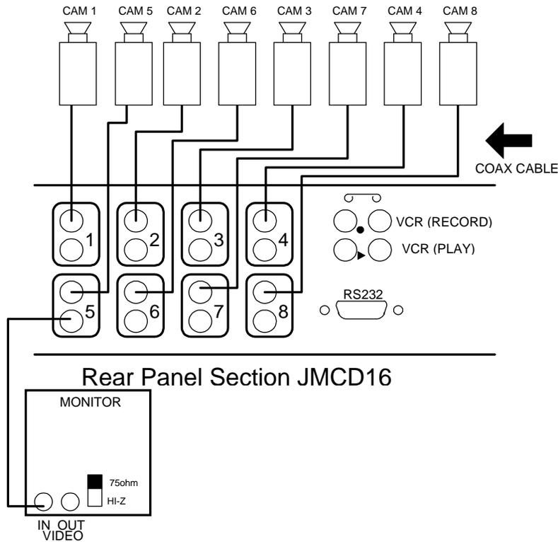
**Figure 1.4 Terminating The Video Signal With A 75ohm Load - JMCD16**
