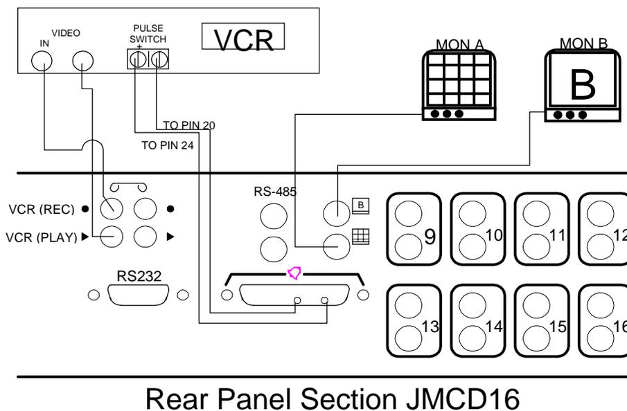
**Figure 4.2 Connecting VCR - JMCD16**
