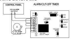
JP1 = MIN -Adjust R3 to SEC, then switch to MIN.
