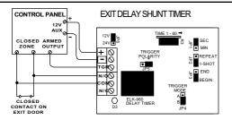
Jumper Settings = SEC or MIN -Adjust R3 for desired delay time.
