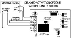
JP1 = SEC -Adjust R3 for desired delay time Jumper
