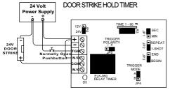
JP1 = SEC -Adjust R3 for desired delay time Jumper
