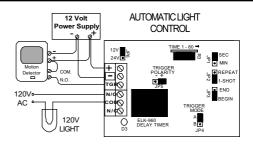
Jumper JP1 = SEC or MIN -Adjust R3 for desired delay time.
