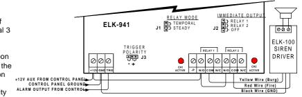
As shown, this hookup is used to activate an ELK-100 siren Yelp sound on Relay 1 from a steady alarm output and a Temporal 3 pulse sound on Relay 2 from a pulsing alarm output. Relay 2 will also activate immediately during the 3 to 4 second verification time delay (regardless of a steady or pulsing input trigger). This immediate output feature is good if the control does a siren test at arm or disarm time.
