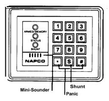
The face of the keypad lifts up to reveal a convenient index of protected zones.
