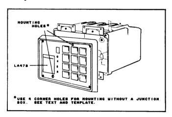
RP854 Keypad in RPB-2 Double-Gang Box (front panel of keypad omitted for clarity).
