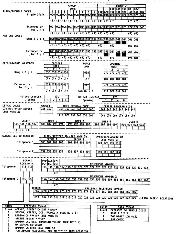
NOTES: (1) 2-DIGIT FORMAT ONLY. (2) DEALER & USER PROGRAM CODES MUST NOT START WITH THE SAME NUMBERS. (3) GROUP-2 CODES MUST BE ENTERED, EVEN IF THEY ARE THE SAME AS GROUP-1 CODES. (4) MUST BE PROGRAMMED IF OPENING/CLOSING CODES ARE PROGRAMMED. (5) THESE FORMATS TYPICALLY USE A 2300Hz HANDSHAKE; ADD AN "8" TO THIS ENTRY. PF171 10/91
