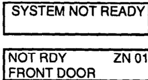
In this example, the front door is not ready (Zone 1). In order to make the system ready determine which zones are not ready by observing the zone indicator lights, or the display section of the LCD keypad. From the zone number you can find out which area of protection is not ready. For example, assume the zone 1 is not ready. Typically, this might mean that a protected door or window is open.
