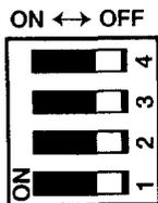
The receiver's DIP switch must be set for a device address of "0", as described in its instructions (all switches to the RIGHT... "off").
