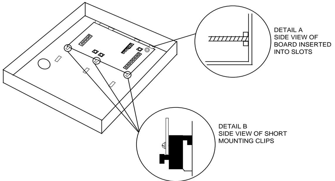
**Figure 4-3: Mounting the PC Board**
