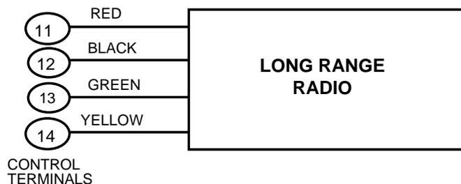
**Figure 13-1: Long Range Radio to Keypad Terminals**
