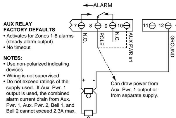
**Figure 15-1: Auxiliary Relay Used as Unsupervised Bell Output**
