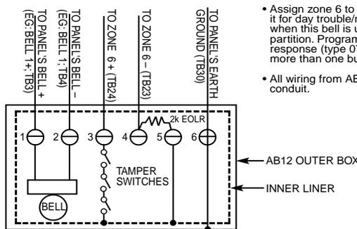
**Figure 14-1: External Sounder Connections**
