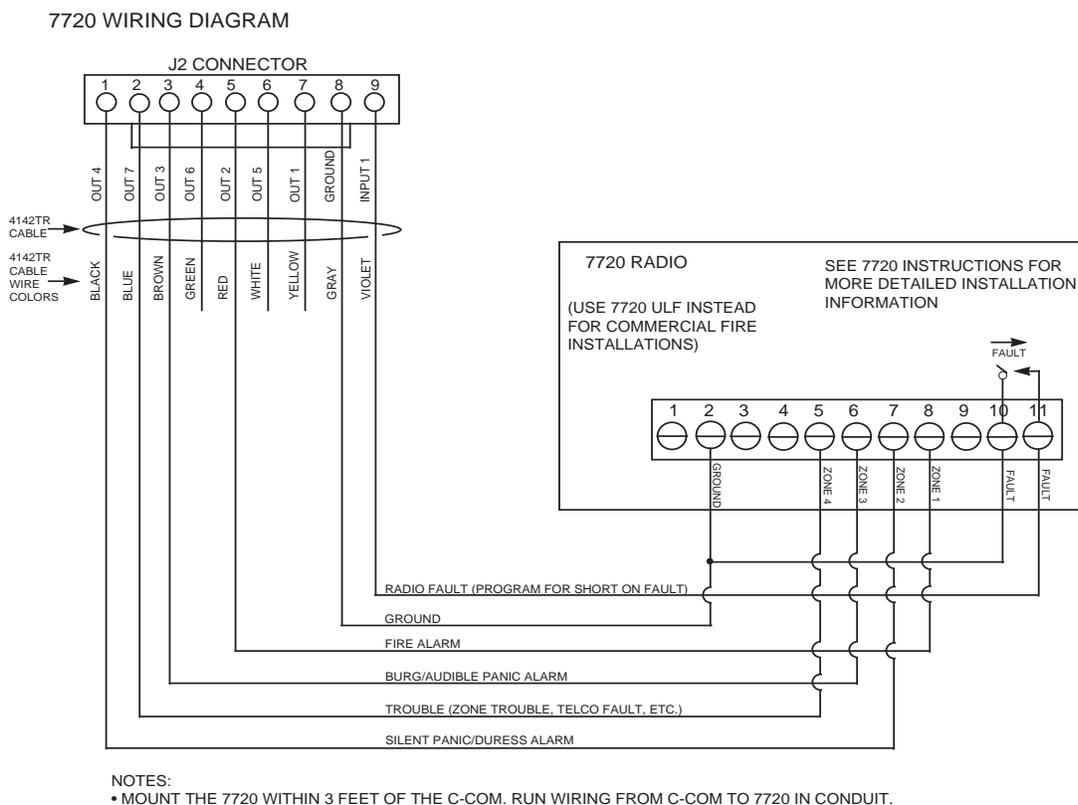
**Figure 12-5a: Connections to 7720 Long Range Radio**
