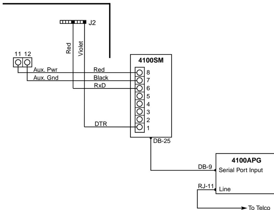
**Figure 18-1: Wiring the 4100APG Without the Serial Printer**
