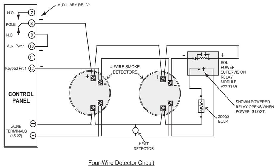
**Figure 15-2: Auxiliary Relay Used for Resetting 4-Wire Smoke Detectors**
