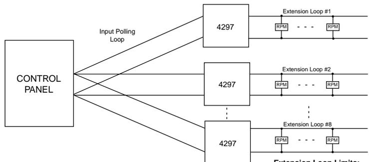
Up to 8 modules may be connected in parallel. Extension loops will be electrically isolated if blue jumper on each 4297 is left intact.
