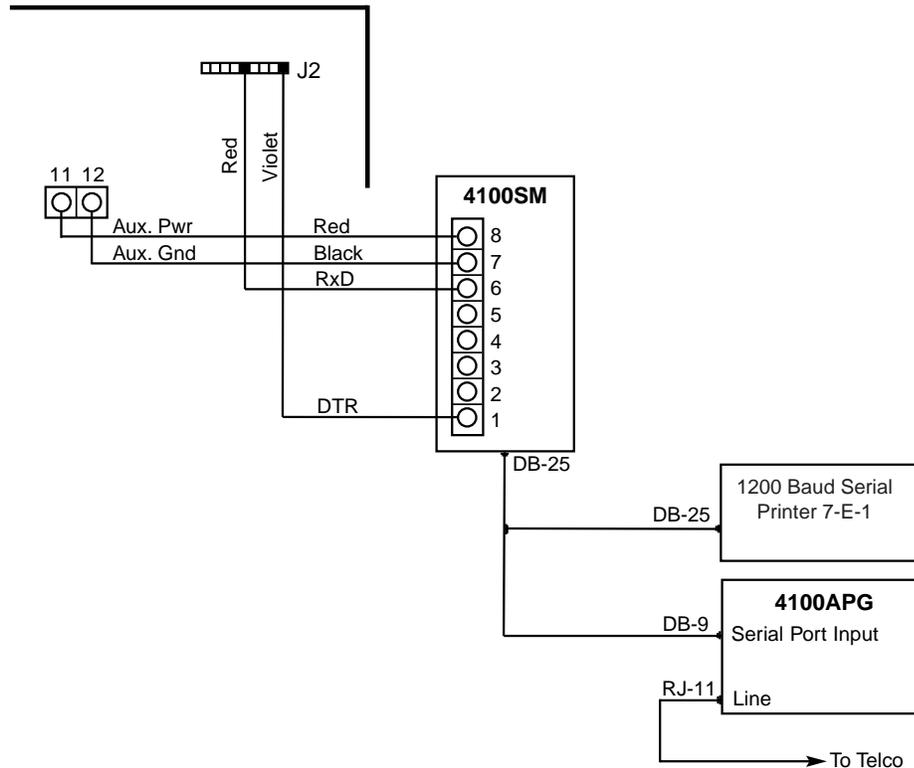
**Figure 18-2: Wiring the 4100APG With the Serial Printer**
