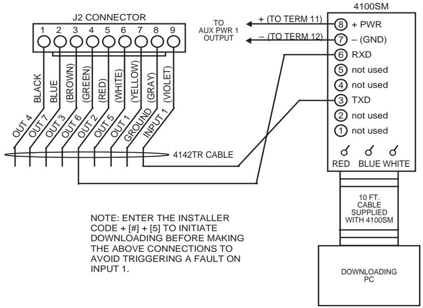
**Figure 25-1: Direct Wire Downloading Connections**
