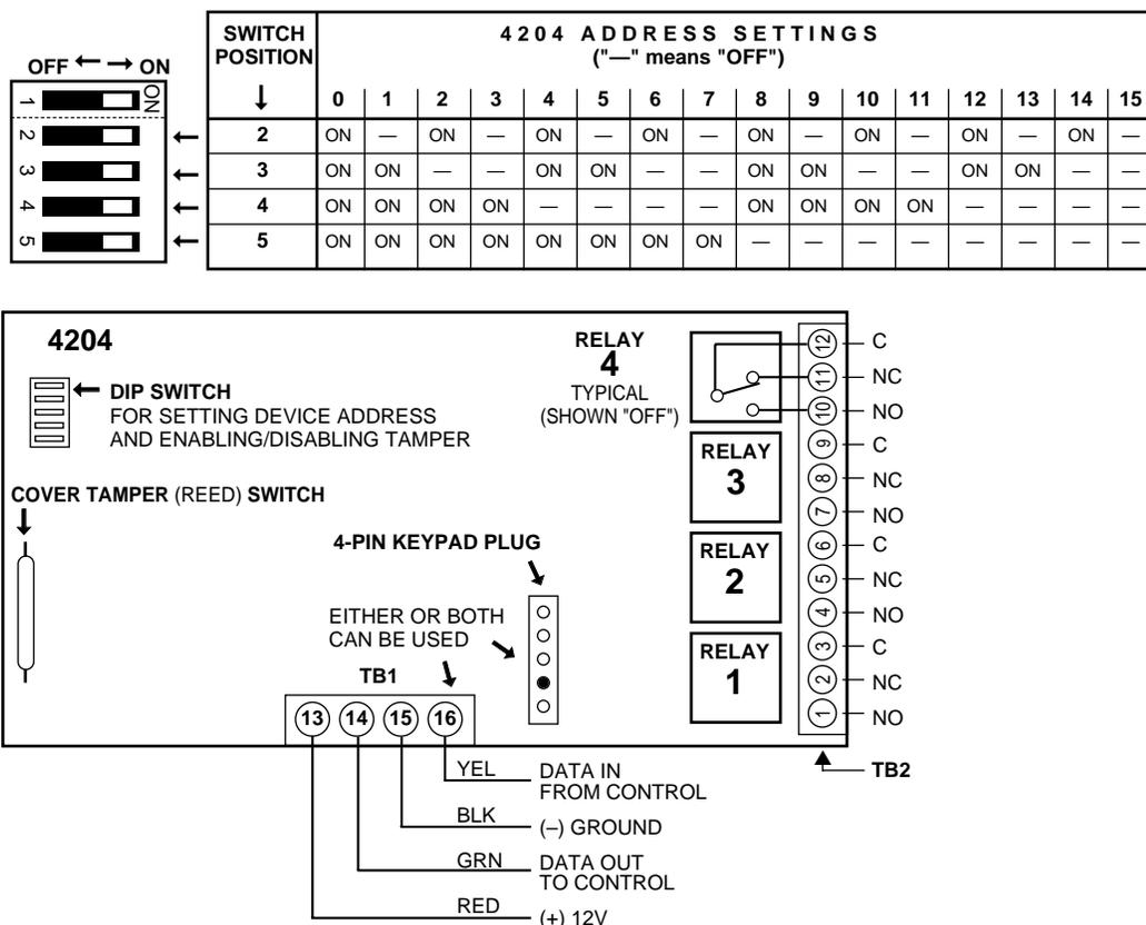
Figure 9-1a: 4204 Relay Module
