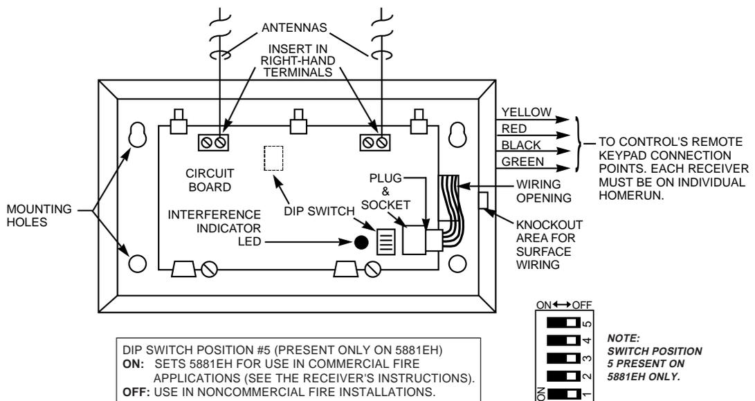
**Figure 8-1: 5881 RF Receiver (cover removed)**
