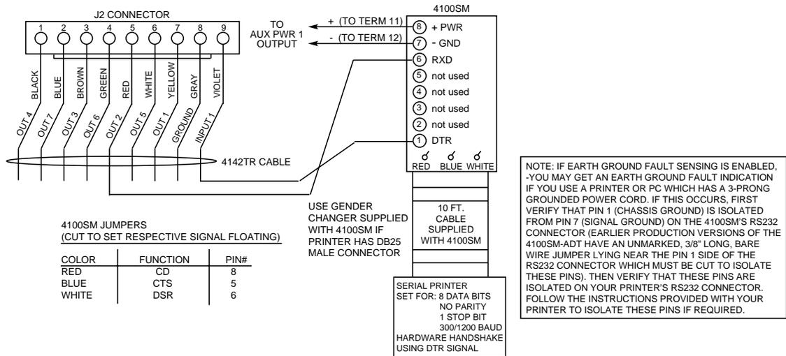
Figure 17-1: Event Log Printer Connections
