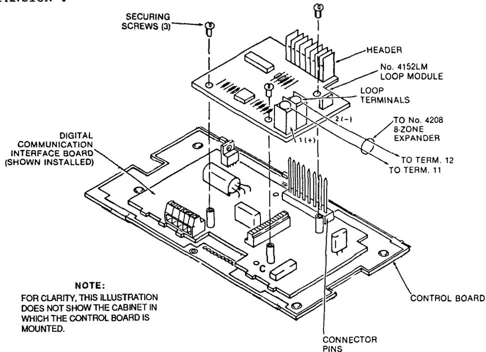
**Diagram 3: No. 4152LM INSTALLATION AND WIRING TO No. 4208**
