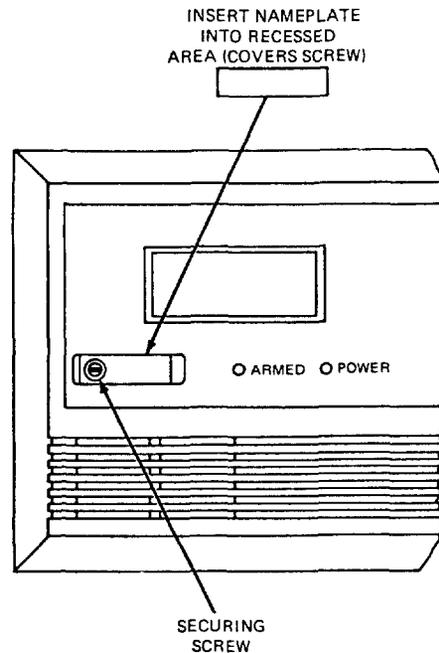
**Diagram 4. INSERTING NAMEPLATE**
