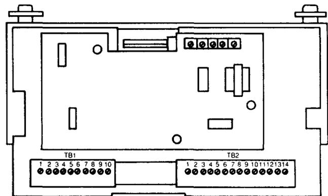
FUSES LOCATED ON UNDERSIDE OF CIRCUIT BOARD (VIEW A)
