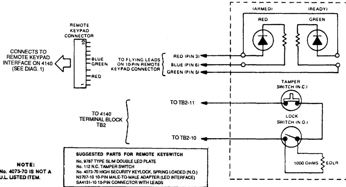
Diagram 2. KEYSWITCH WIRING
