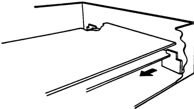
Remove the board by sliding it away from the slotted mounts.
