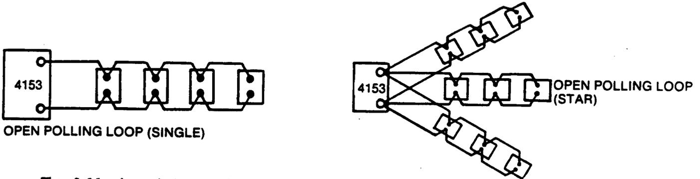
The following wiring configurations are used with the addition of the 4152LM.
