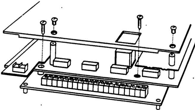
Remove lower cover and circuit board mounting screws.
