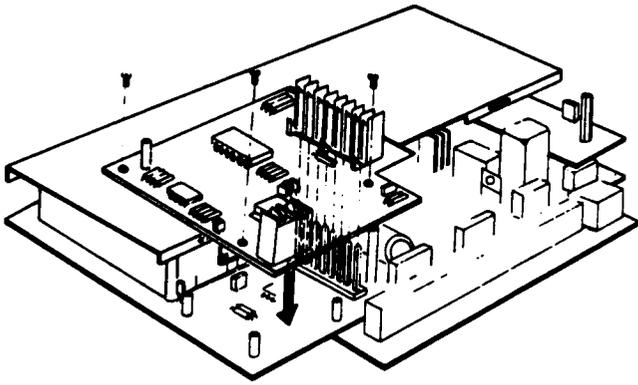
Install the 4152LMB by carefully inserting the square post connectors into the header. Take care not to insert the posts too far. Replace the lower circuit board cover.
