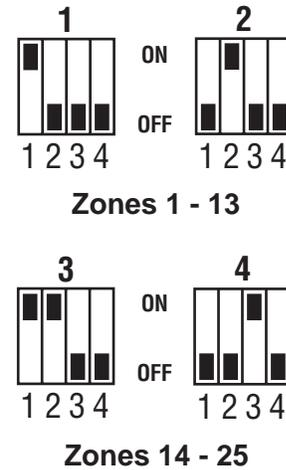
Figure 3.8 2500-RA/RADVR Address Switch Settings
