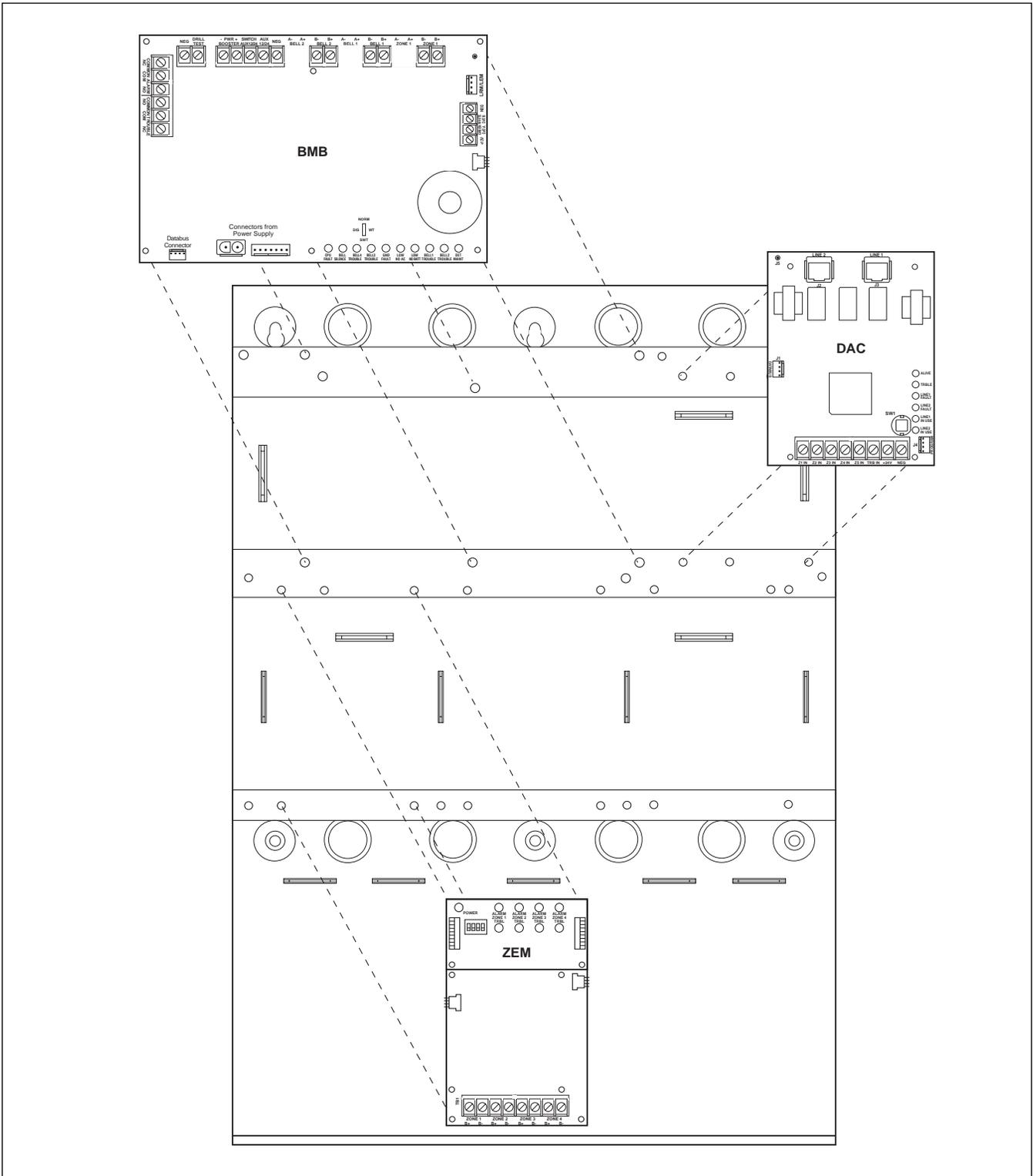
Figure 3.10 ZEM, BMB, and DAC Installation Diagram
