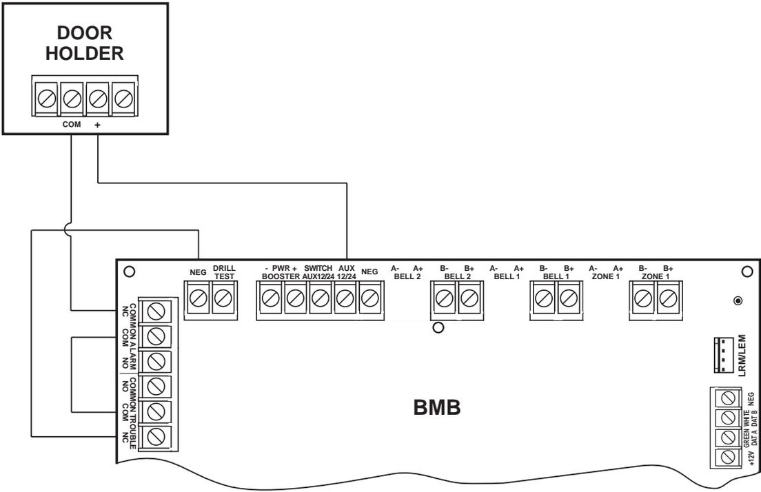
**NOTE:** Program common trouble contacts for open on loss of AC. See Section 5.0 *Programming*.
