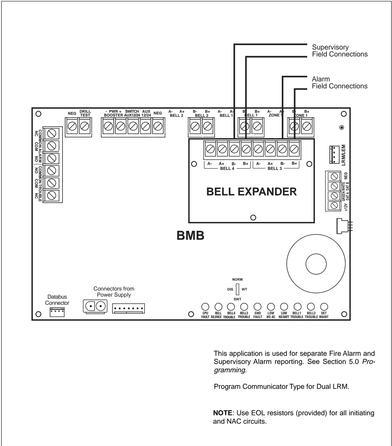
Figure 2.10 Dual LRM Installation Diagram
