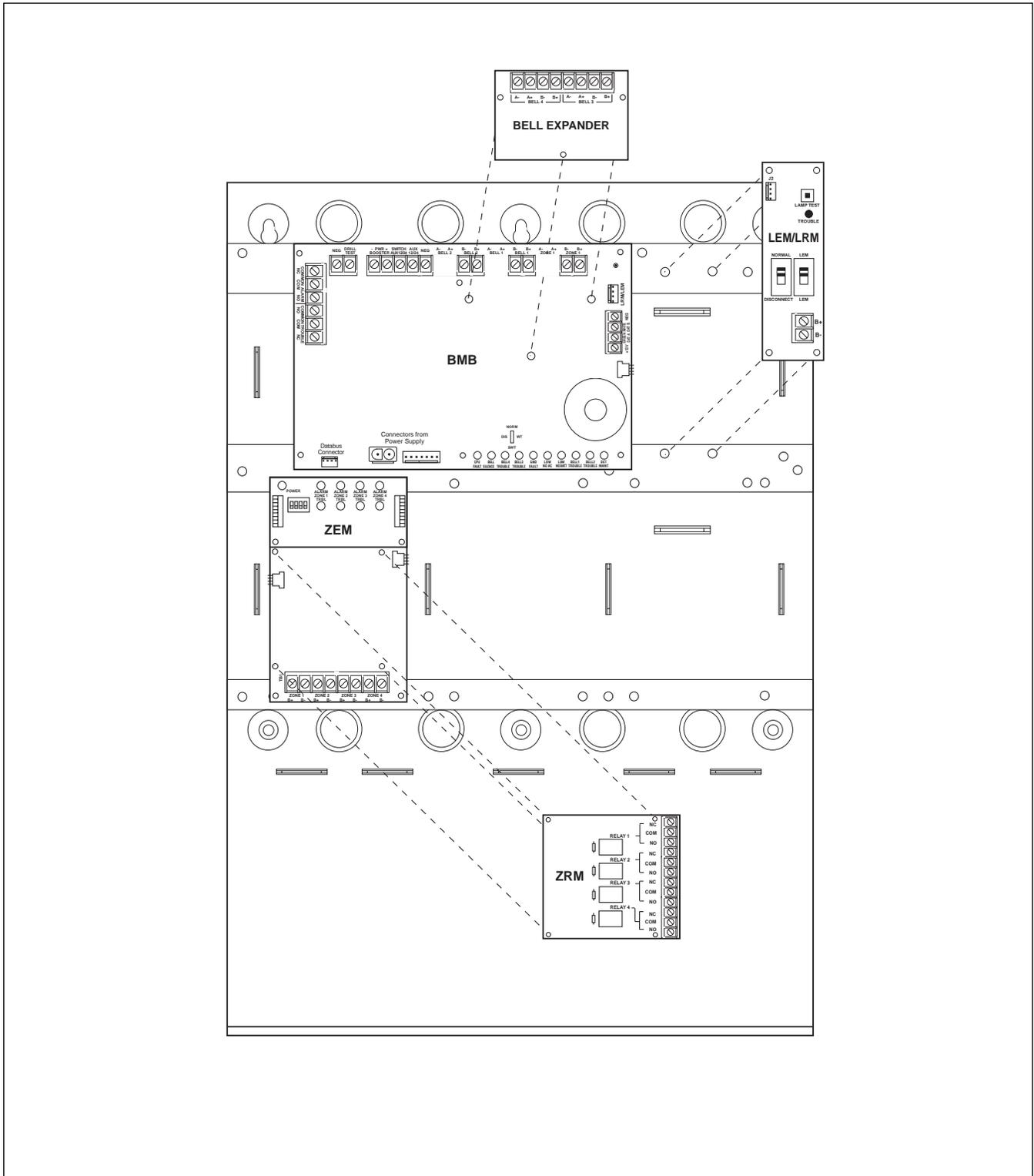
Figure 3.11 BELL, ZRM and LEM/LRM Installation Diagram
