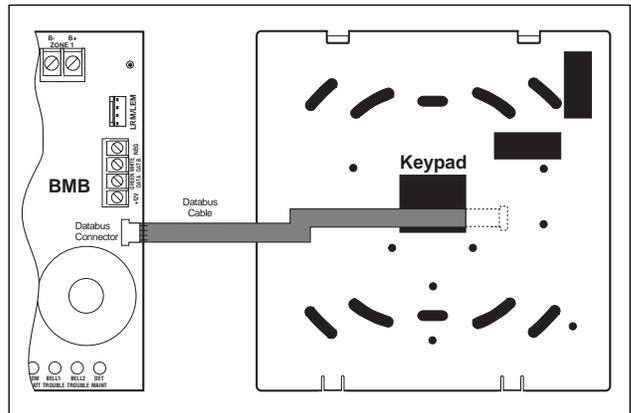
Figure 3.5b Connecting BMB to Keypad
