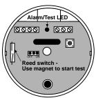
test period is over. The test mode can be restarted at any time by powering the unit off and then on or by placing a magnet next to the "T" on the cover. Placing a magnet next to the "T" when the unit is in the test mode will terminate the test.
