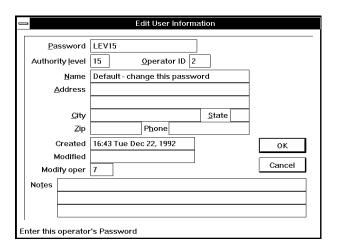
From this window you may enter and edit all necessary information. Some fields are filled-in automatically by WDSRP: the Operator ID field, Created Field, Modified field, and the Modify Operator field.
