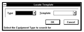
Fill-in the Equipment Type field (if known) and select O.K. The Templates with that Equipment Type will now be available to scroll through (scroll through the Template database by using the commands at the bottom of the window: Beginning, Previous, Next, and End of File).
