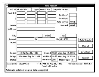
AUTOMATIC UPDATE: This command will update all data as needed. **CAUTION:** The automatic update command will make changes based on the most current information in either the Account or the control panel. When you first contact a control panel, you should first perform a complete upload or download.
