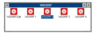
The WDSRP Edit icon is used for editing purposes only. It does not communicate with the control panels. Use this selection when work needs to be done to any of the WDSRP databases, but communication to a control panel is not necessary.
