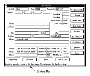
In the example above, the Locate Key is highlighted and the Status Bar explains that the Locate Key will locate a specific record in the database.
