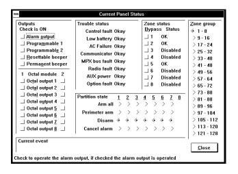
The Status command will call up the Current Panel Status window. This window will show you the status of system parameters specific to this Account/control panel such as: zone status, output status, trouble status, arming state, partition state. You may also edit the status of the control panel from this window.
