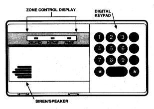
**INSTANT** — When this green indicator is lighted, the instant area is ready to be armed. When the INSTANT indicator is not lighted, the area is not ready to be armed (check doors, windows, and motion detectors in the instant area). Both the DELAYED and INSTANT indicators must be lit before arming.
