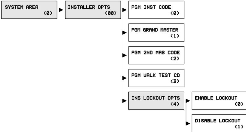
SYSTEM AREA (0) ▶ INSTALLER OPTS (00) Scroll to desired option using the [<][>] keys and press [\*].
