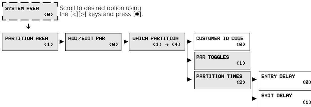
Using the first method the arrow keys would have to be pressed many times to scroll to the various items followed by the [\*] key to select the item. Twelve keystrokes would be required after entering Installer Programming providing no mistakes are made. The keystrokes required are as follows:
