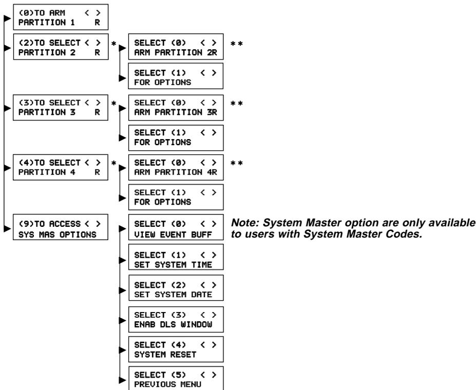
\* These partitions will only be displayed if the partition is enabled and the access code is assigned to that partition. The partition status indication on the lower right corner of the display will change according to the status of the partition.
